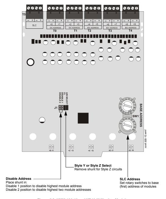
Figure 5.2 NMM-100-10 and XP10-M Monitor Modules
