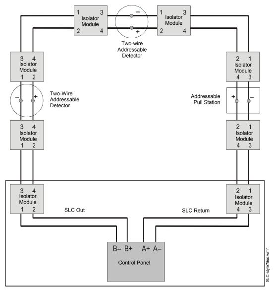
Figure 4.6 NFPA Style 7 SLC Using Isolator Modules
