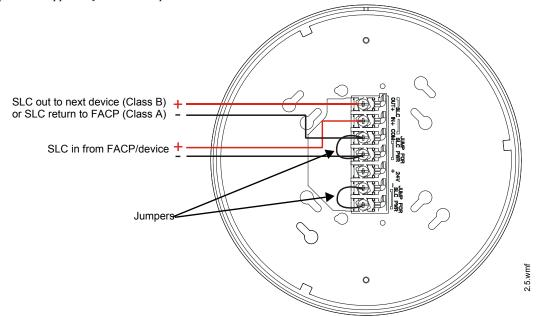
Figure 8.6 FWSG Powered by the SLC
