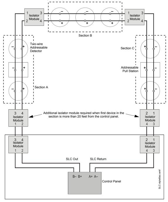
Figure 4.5 NFPA Style 6 SLC Using Isolator Modules
