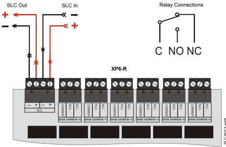
Figure 7.3 XP6-R Wiring Connections
