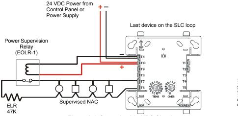
Figure A.1 Supervised 24 VDC Circuit
