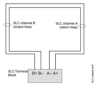
Figure 2.4 Measuring the Wire Length - Four-Wire SLC
