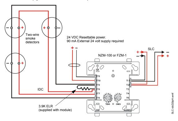
Figure 5.16 Typical Style D IDC Wiring with an NZM-100 or FZM-1
