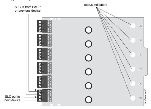
Figure 4.2 Wiring an ISO-6 Module
