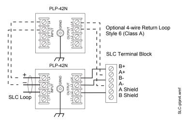
**NOTE:** Use 12AWG (3.25mm2) to 18AWG (0.75mm2) wire with crimp-on connectors to connect the unit's ground terminal to equipment ground. Wire length must be minimized to provide best protection.
