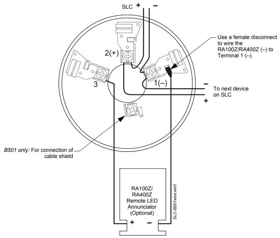
Figure D.1 Wiring the Legacy B710LP or B501 Detector Base
