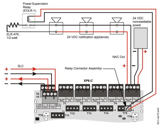
Figure 6.5 NFPA Style Y Notification Appliance Circuit
