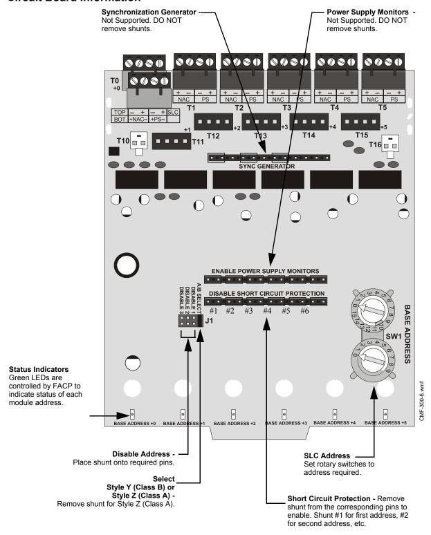
Figure 6.4 XP6-C Control Module Settings
