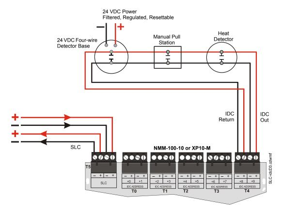
Figure 5.13 Typical Style D IDC Wiring with an NMM-100-10 or XP10-M
