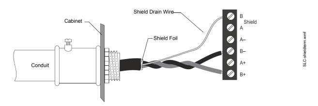
Figure 2.5 Shield Termination
