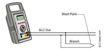
Figure 2.1 Measuring DC Resistance of a Two-Wire SLC
