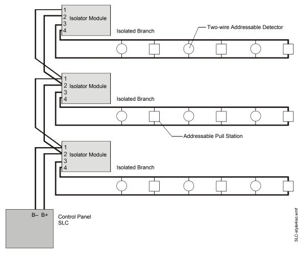
Figure 4.3 NFPA Style 4 SLC Using N100-ISO and ISO-X Isolator Modules
