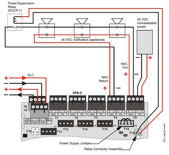
Figure 6.6 NFPA Style Z Notification Appliance Circuit
