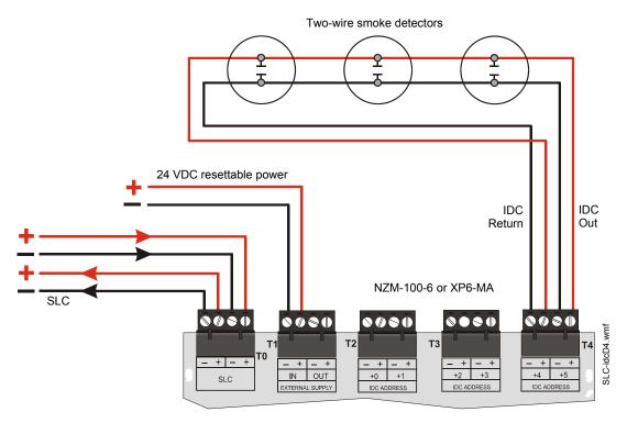
Figure 5.18 Typical Style D IDC Wiring with an NZM-100-6 or XP6-MA
