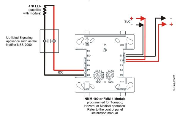
Figure 5.11 Emergency Signaling Wiring with an NMM-100 or FMM-1
