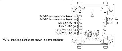
Figure 6.1 NC-100 and FCM-1 Wiring Connections
