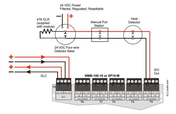
Figure 5.12 Typical Style B IDC Wiring with an NMM-100-10 or XP10-M
