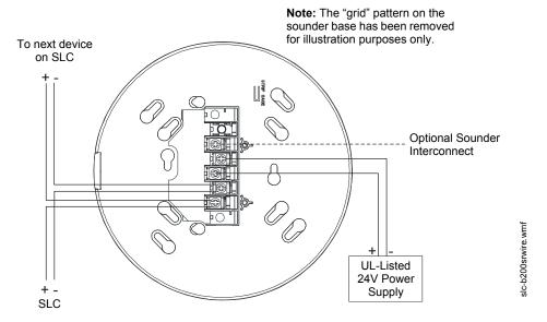
Figure 8.4 Wiring of a B200S(R)/B200S(R)-LF Sounder Base
