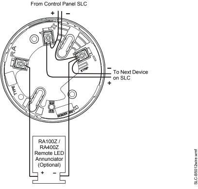
Figure 8.1 Wiring a B300-6, B210LP, or B501 Detector Base
