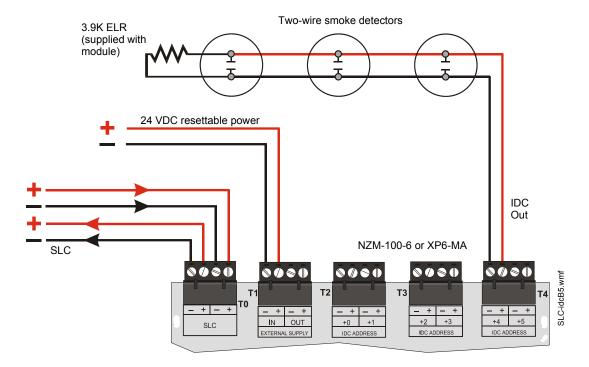
Figure 5.17 Typical Style B IDC Wiring with an NZM-100-6 or XP6-MA
