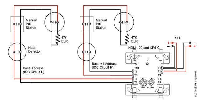
Figure 5.14 Typical Style B IDC Wiring with an NDM-100 or XP6-C
