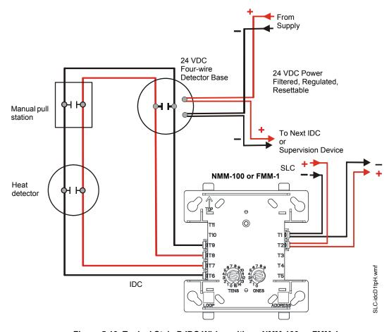
Figure 5.10 Typical Style D IDC Wiring with an NMM-100 or FMM-1
