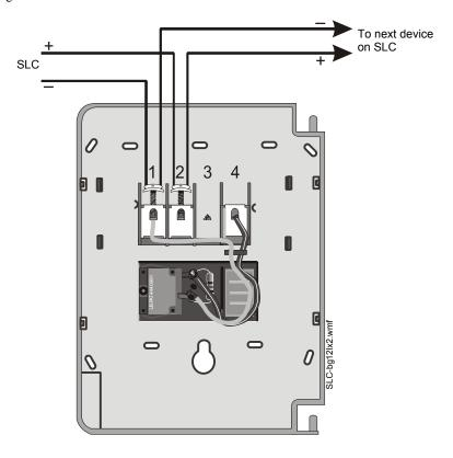
Figure 10.1 Wiring of a NOT-BG12LX and NBG-12LX Pull Station to an SLC
