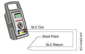
Figure 2.3 Measuring DC Resistance of a Four-Wire SLC
