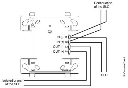
Figure 4.1 Wiring N100-ISO and ISO-X Modules
