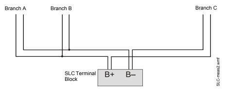
Figure 2.2 Measuring the Total Wire Length - Two-Wire SLC
