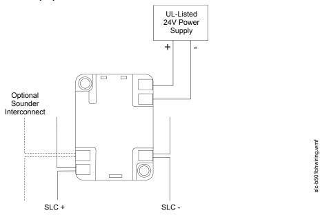
Figure D.4 Wiring the Legacy B501BH(-2) and B501BHT(-2) Sounder Bases
