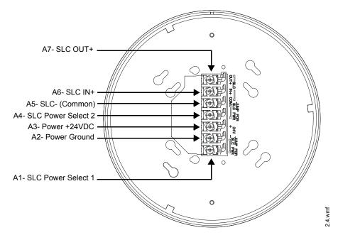
Figure 8.5 FWSG Mounting Plate - Terminal Layout
