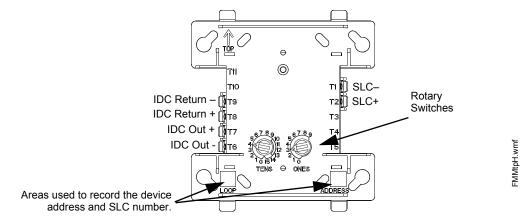
Figure 5.1 NMM-100 and FMM-1 Monitor Modules
