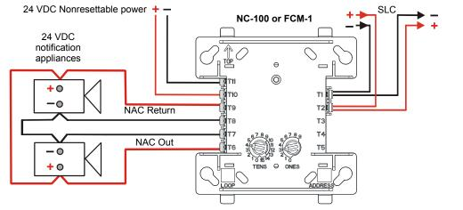
Note: Module polarities are shown in alarm condition.
