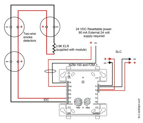
Figure 5.15 Typical Style B IDC Wiring with an NZM-100 or FZM-1
