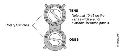
Figure 5.8 Setting an SLC Address on a Multi-Point Module
