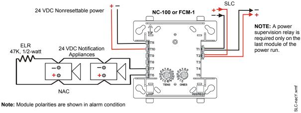
Figure 6.2 NFPA Style Y Notification Appliance Circuit
