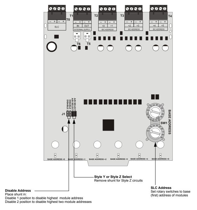
Figure 5.4 NZM-100-6 and XP6-MA Interface Modules
