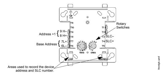
Figure 5.5 NDM-100 and FDM-1 Dual Monitor Modules
