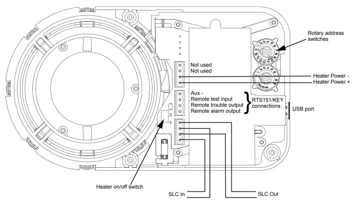
Figure 9.1 FS-OSI-RI Beam Detector Terminal Block Wiring
