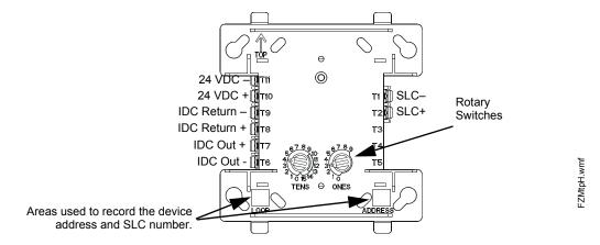
Figure 5.3 NZM-100 and FZM-1 Interface Modules
