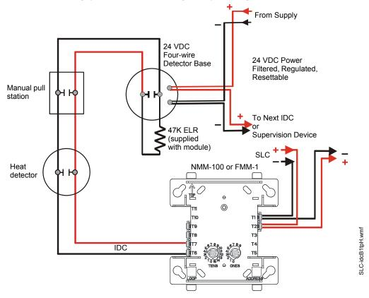
Figure 5.9 Typical Style B IDC Wiring with an NMM-100 or FMM-1
