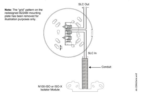
Figure 8.2 Wiring of a B224BI Isolator Base Mounting Plate
