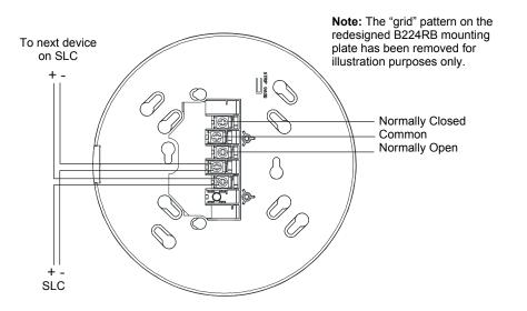
Figure 8.3 Wiring of a B224RB Relay Base Mounting Plate
