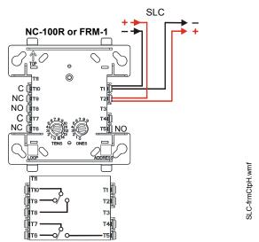
Figure 7.1 NC-100R and FRM-1 Wiring Connections
