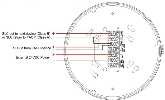
Figure 8.7 FWSG Powered by a Regulated, External Source
