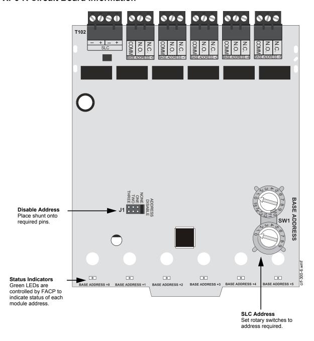
Figure 7.2 XP6-R Control Relay Module
